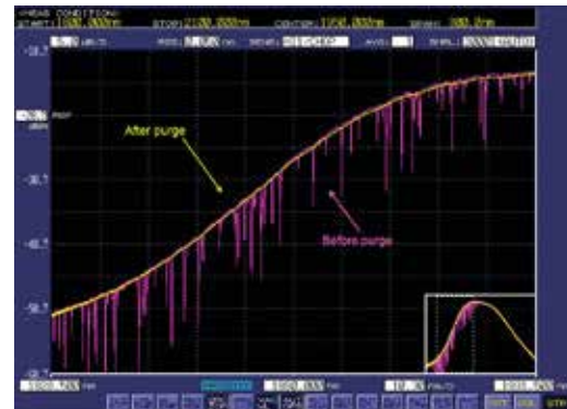
Effect of purging (dry-air, 1 hour) water vapour absorptions around 1900 nm.
