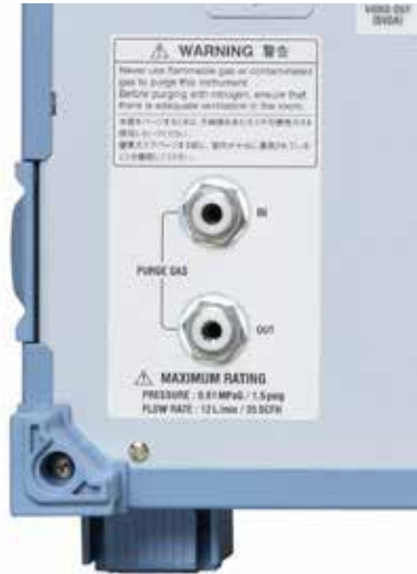
Purge gas ports on the Yokogawa AQ6375B optical spectrum analyser
