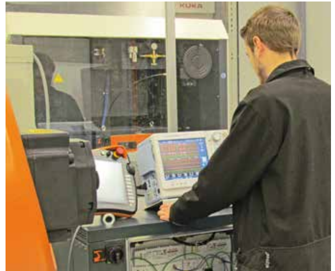
Tobias Zimmermann (KUKA Systems) measures the power consumption of the robot with the Yokogawa PX8000 Precision Power Scope.
