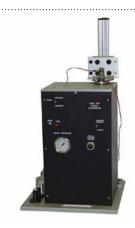
The Endevco® model 2925 POP provides an accurate and controlled means of shock sensitivity calibration of accelerometers by using the model 2270, a back-toback comparison calibration standard accelerometer. Calibrations are performed at accelerations from 10 g to well above 10 000 g at half-sine pulse durations from 3 ms to 100  $\mu$ s. The system can be used manually in a stand-alone mode, or in a fully computer controlled mode.
