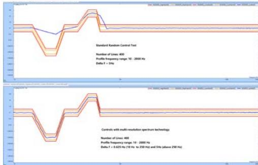
Obviously, the one with multi-resolution can achieve much better control dynamic range than that of without. It is common to see a 20dB or more improvement of the control dynamic range in the low frequency range.
